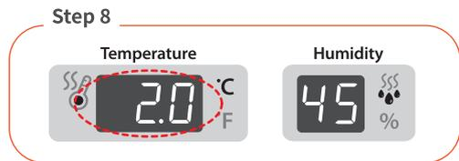
ex : ※ It shows that the set temperature value is approximately 3°C (3°F) higher than the actual cabinet temperature of the machine.
